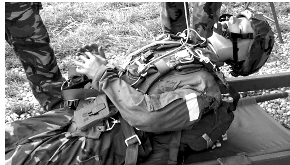
Figure. Instrumented manikin configured with T-10 parachute and LW-V1.0 helmet.
